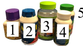
Fig. 3: Bottles used in experiments with different safety mechanism: (1) push-and-twist , (2) pinch-and-twist , (3) push-and-twist , and (4) push-and-twist . (5) Bottle with no safety mechanism.
